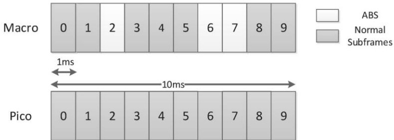
Figure 4.2 ABS in multi-tier heterogeneous cellular networks scenario. SOURCE: Reproduced with permission from [23]. Copyright 2015 Springer International Publishing.
