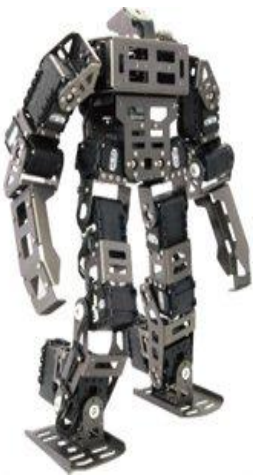
Figure 1.6 Smart Humanoid ver 2.0 using embedded system and webcam based on LINUX Ubuntu.
